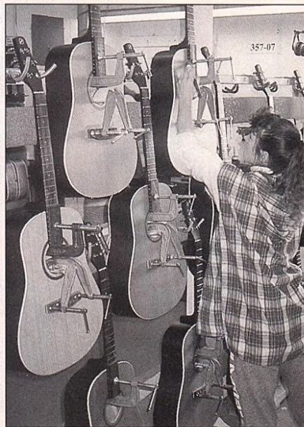
A La Si Do employee oversees the gluing of bridges and fingerboards.
