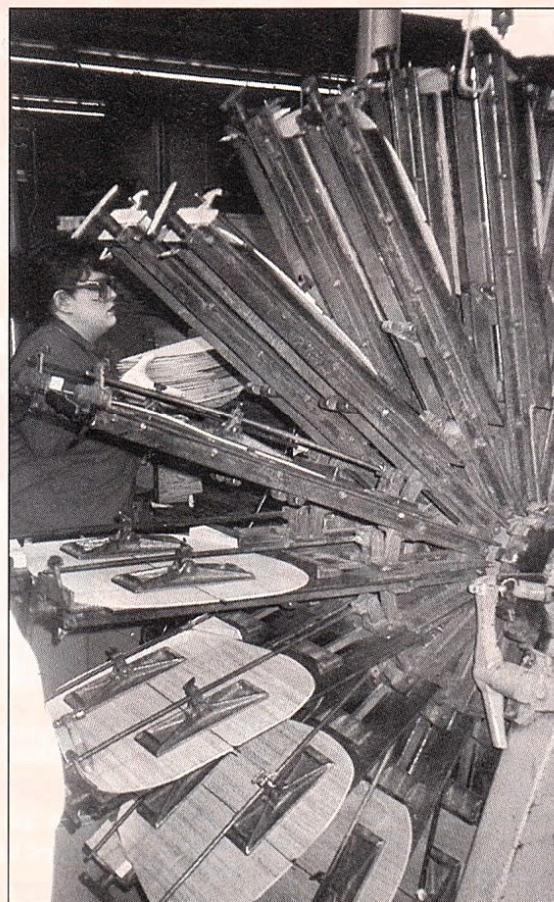
Martin has used this paddlewheel to glue tops and backs since the '30s.
