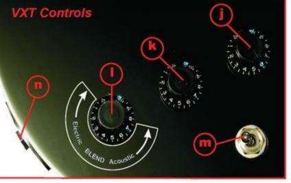
Pickup Volume Control adjusts the output level of all pick-
