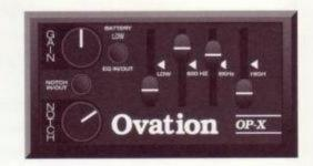
The OP-X features four precise bands of EQ (at 80Hz, 600Hz, 6.6KHz and 10KHz) to contour the sound accurately plus a very steep (30dB/octave) notch filter designed to kill feedback one note at a time. Now you can solve feedback problems without changing the character of the sound.
