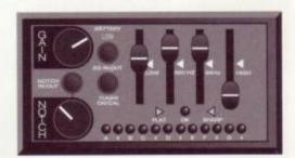
The Optima uses the latest generation of analog electronics, giving the system noise specs comparable to recording studio consoles (-104.3dB). The Optima also features a highly accurate on-board chromatic tuner for standard, open or non-standard tunings.
