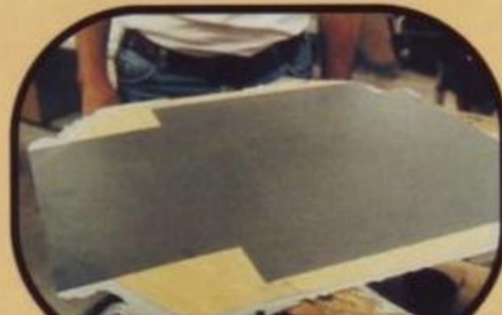
7) Adamas composite top ready for shaping. A thin birch centre laminate flanked by epoxy-impregnated veneers of textured graphite 'tape' give a thickness one-third that of conventional all-wood tops, combining lateral flexibility with lengthways stiffness.
