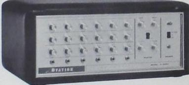
Public Address Specially designed for vocal. Six channels; bass, treble and volume control on each with reverb selective by pulling volume knob. Master panel; master volume, bass, treble, reverb, and reverb on/off switch. Stereo facility; 3 channels left, 3 right; or monaural. Line reversal switch.
