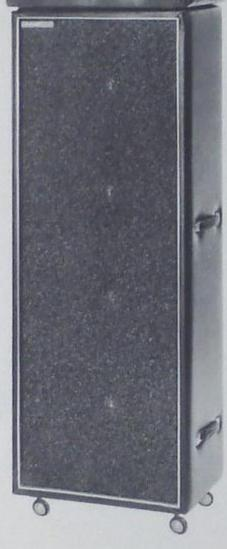
Can be used for either public address or music reproduction. 60" high, 22" wide, with four 12" Ovation speakers, or 50" high, 18" wide with four 10" Ovation speakers. With or without built-in 100 watt power amplifier. Designed for use with Ovation public address preamp.
