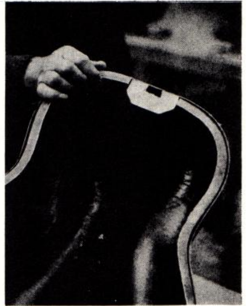
WOOD TOP IS BONDED to Lyracord body in the same way that Kaman helicopter blade employing wood, Lyracord and metal is made.
